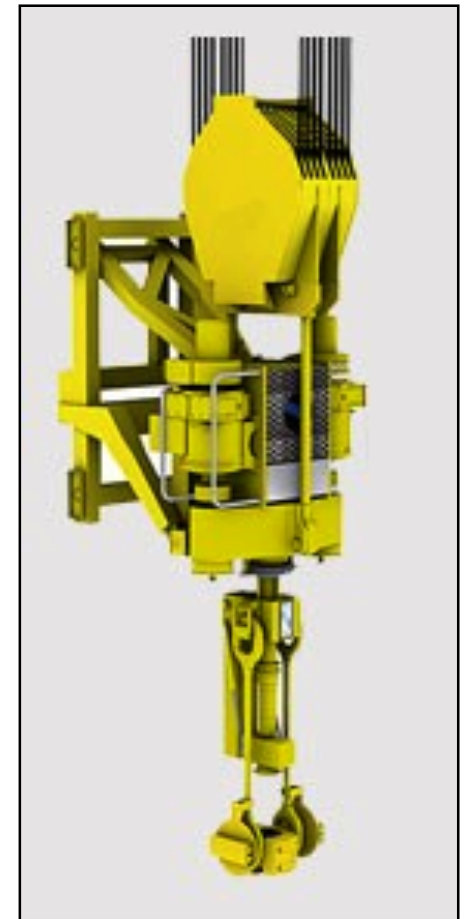
Fig. 1 Images of ship-mounted crane at sea state 0 and off-shore oil platform with top drive equipment. The top drive for this project was rated for more than 2,000,000 lbf of string weight while meeting all API specifications.
