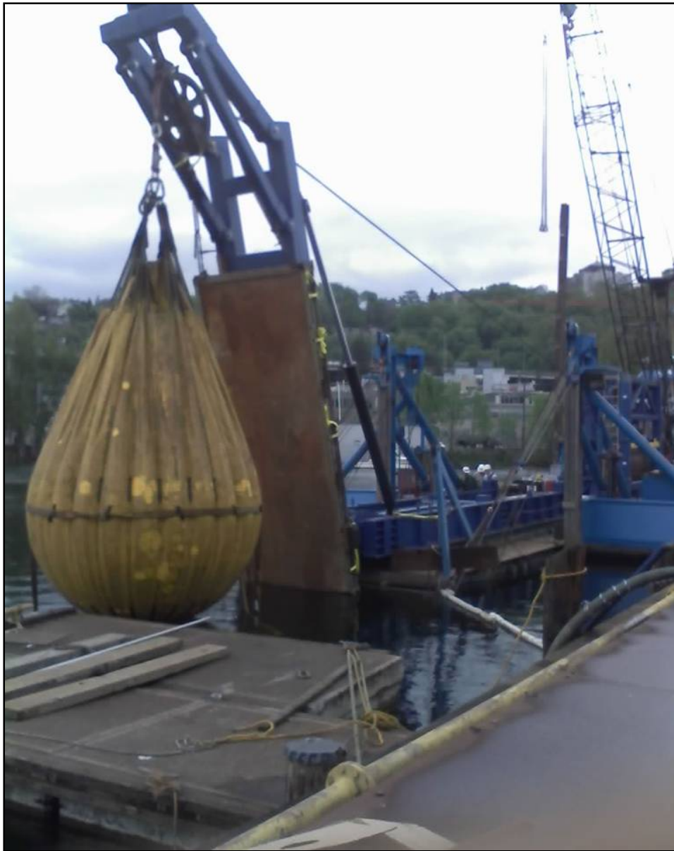
Fig. 4 The crane was field tested using a large water filled bag. It passed with no problems and is now in service somewhere around the world.
