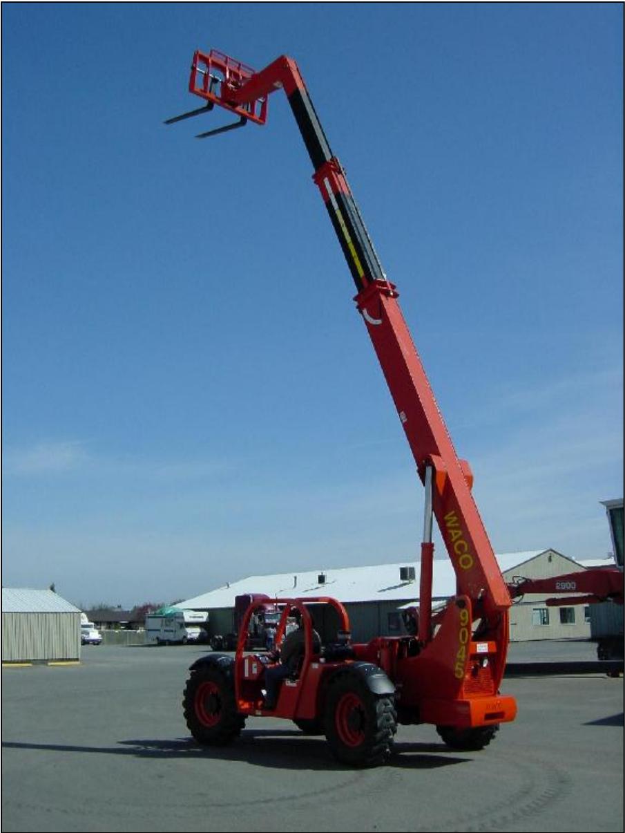
With the boom fully extended, the truck has a reach of 40 ft.
