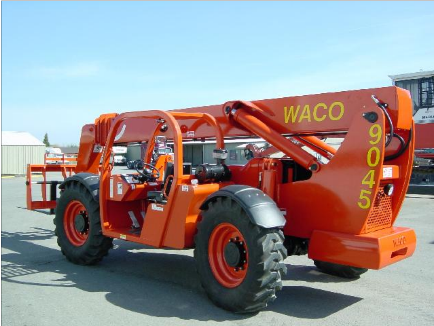
WACO Lift Trucks & Attachments rough terrain telescopic handler. The truck is rated at 9,000 lb lift capacity.
