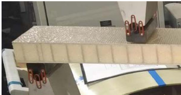
Figure 6 – Experimental work on sandwich laminate composite with FEA comparison
