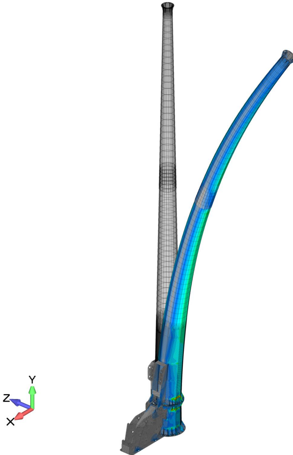
Figure 3: The full tower with exaggerated deformation to illustrate the first normal mode.
