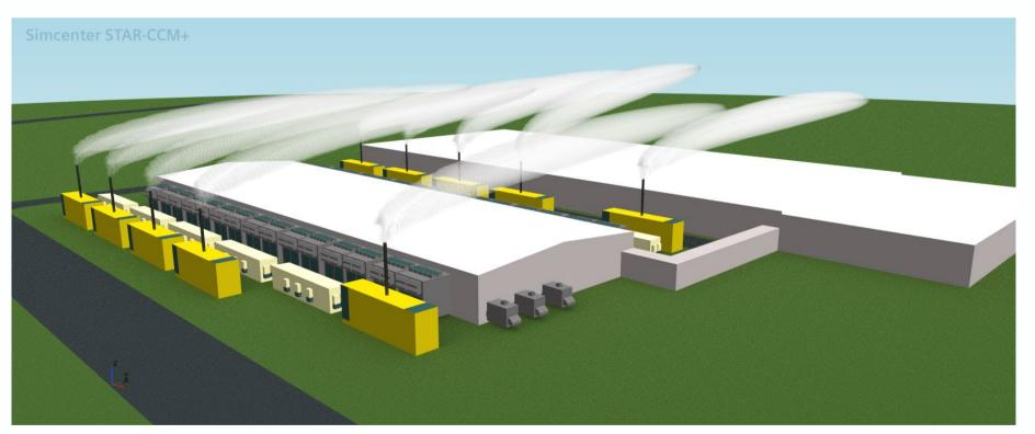
Predictive Engineering has done numerous exterior flow analyses for data centers which are powered by onsite diesel generators. The analyses are performed at different wind conditions to ensure that exhaust and heat from the diesel generators do not contaminate the supply air of cooling equipment into the data center of adjacent buildings.
