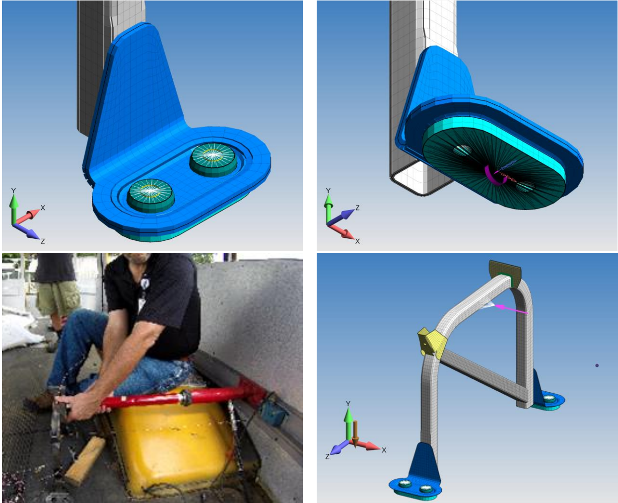
Fig.5: Seat foot / bus floor interface stiffness testing
