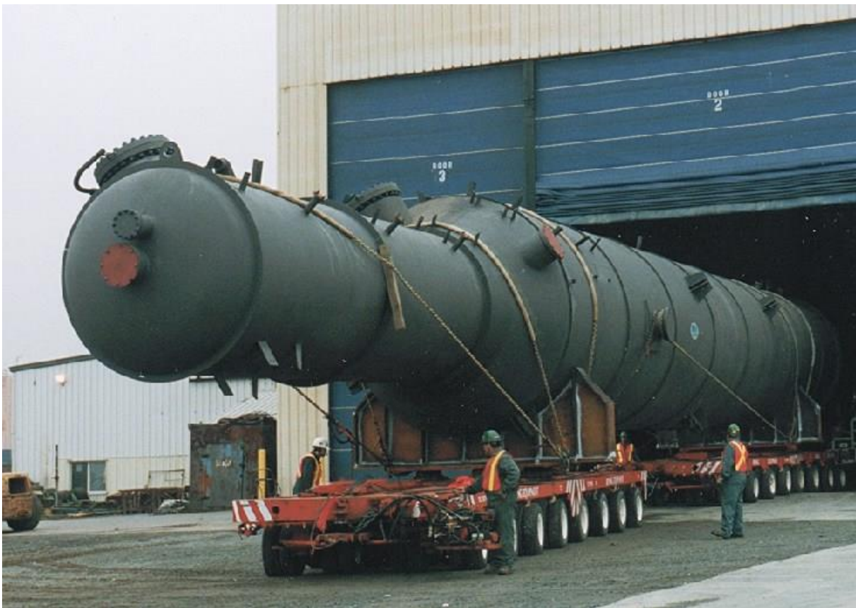
Figure 2: Examples of pressure vessels in transportation. The upper images shows a vessel attached to a schenkel train car. The vessel in the lower image is mounted in saddle supports atop multiple flatbed trailers.
