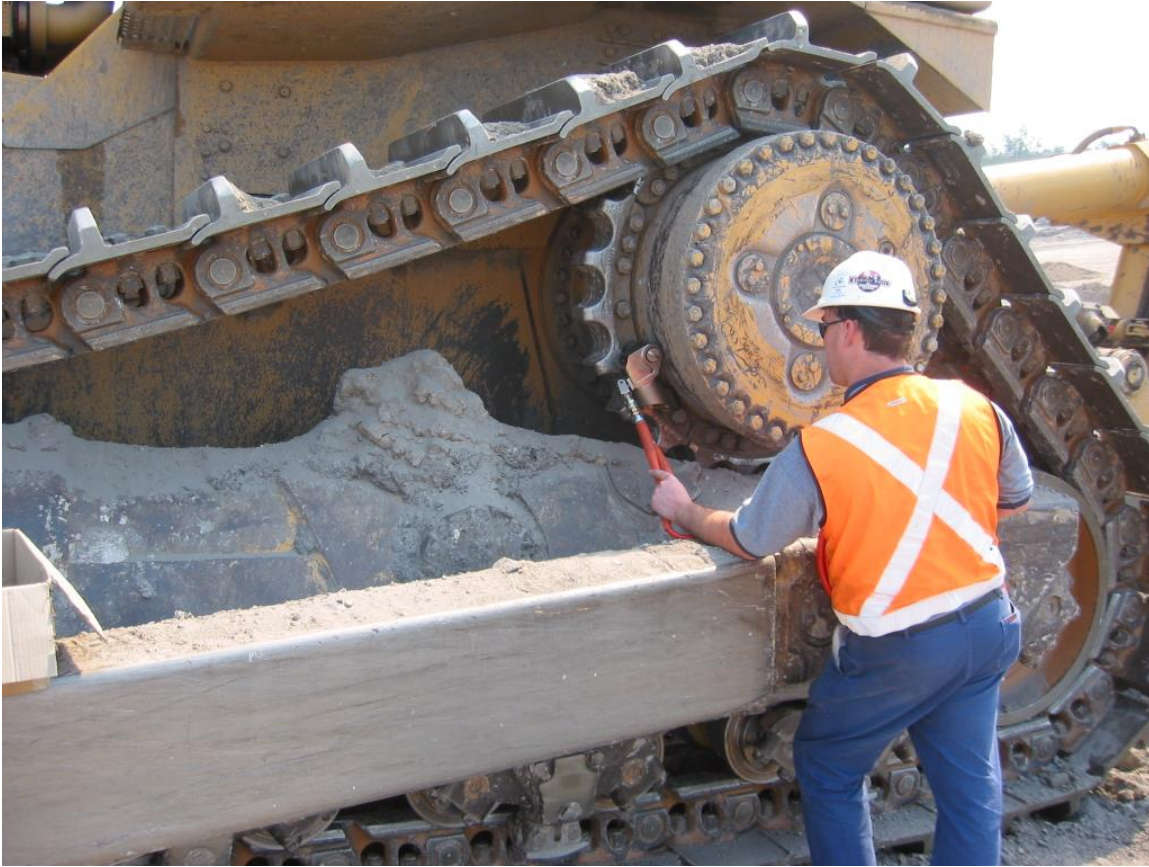
Figure 1: Example of bolted sprocket and hub design on D11 Caterpillar
