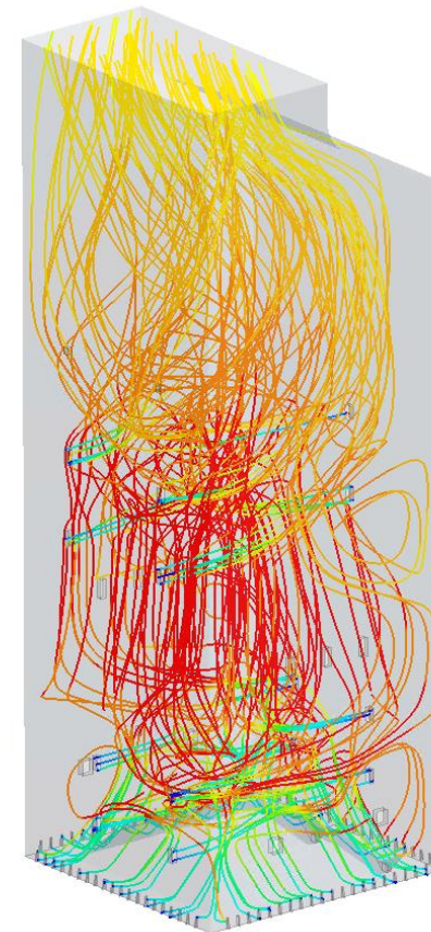
Figure 2: Left: Velocity vector plot (line integrated) of airflow from secondary and tertiary air inlets. Right: Velocity streamlines from main air inlets plotted against air temperatures.
