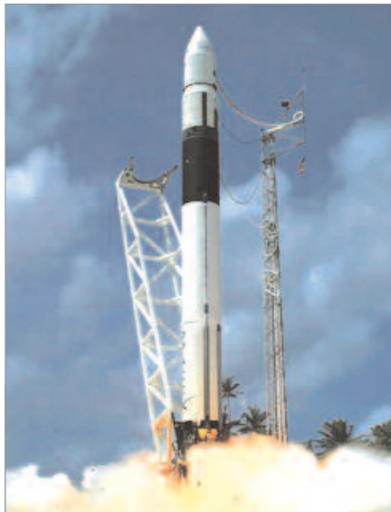
Figure 3a: A rocket launch and other chaotic events create vibration (acceleration) spectra that are best idealized in a statistical sense via power spectral density functions.
