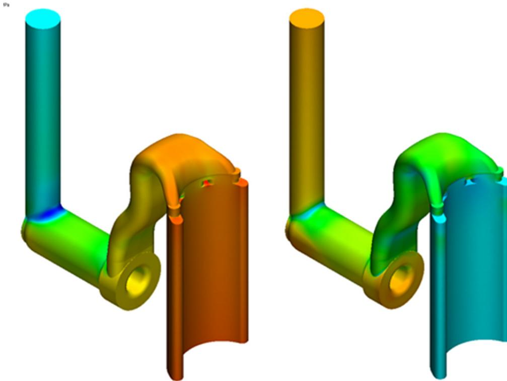
**Figure 2:** The CFD analysis determined the pressure drop for the piston pump in both pump and motor mode. The pressure drop across bends, expansions, constrictions and other discontinuities is dependent on the direction of flow.
