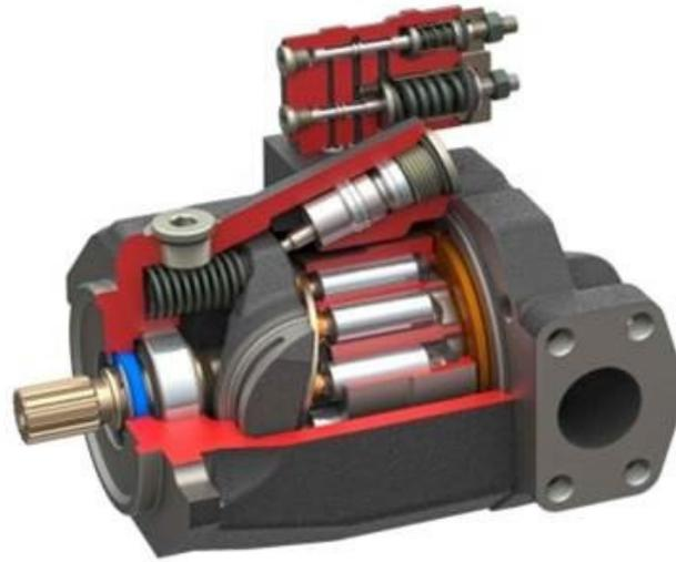
**Figure 3:** A cut-away of an example piston pump shows the internal pistons and swash plate that transfers the hydraulic energy to mechanical energy and vice versa.
