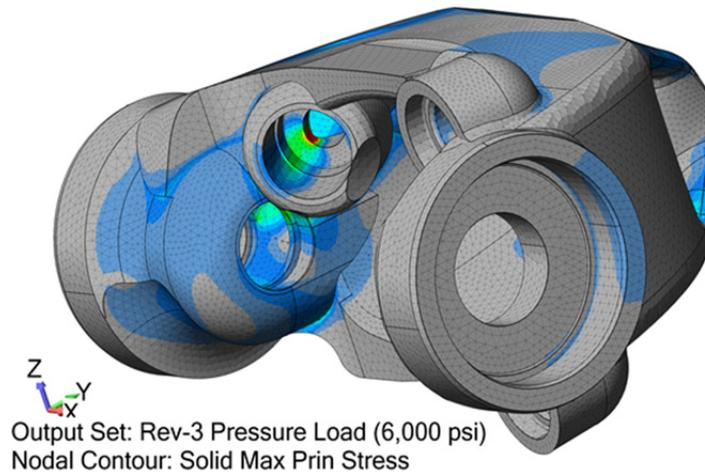
**Figure 4:** Starting with the same CAD geometry, a finite element analysis model was created to calculate stresses generated by the high-pressure hydraulic fluid. The combination of the CFD and FEA models facilitated a design that reduced pressure drop while keeping stresses below code allowables.
