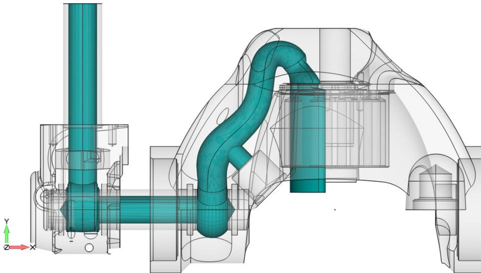
**Figure 1:** The CAD geometry of the piston pump is shown above. The CFD analysis focused on the internal fluid volume shown in green while the FEA focused on the cast structure shown in gray.
